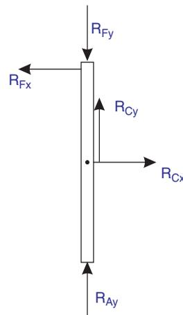
$$R_{Fy} = R_{cy} + R_{Ay} \text{ e } R_{cx} = R_{Fx}$$
